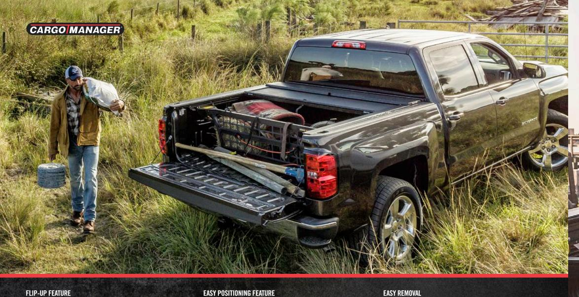
CARGO MANAGER quickly pivots up and out of the way for most loading chores. Its flip-up feature allows the divider to rotate 90 degrees, holding it parallel to, and 12" above, the bed floor. This is accomplished by simply depressing stops located at the ends of each track, rolling the divider back to allow the rear wheels to exit the tracks, rotating the divider 90 degrees and hanging it on the hooks provided. Long objects, such as ladders or lumber, may then be easily loaded under the divider.
