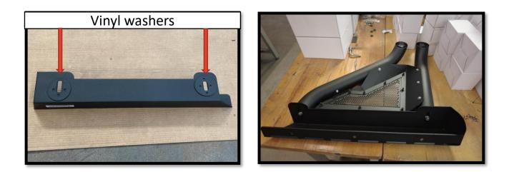
**STEP 5**: Install base plate onto front and rear tubes as shown. Position the rear bottom vinyl washer (item 16) and front bottom vinyl (item 15) in between the tubes and base plate. Fasten down using 3/8" hex bolts (2), 3/8" flat washer (2) and 3/8" lock washer (2). If you're planning on not using a tonneau cover with your Sport Bar, install the base plate cover on the bottom of the rear tube Reference images below. Leave hand tight for later adjustment. Repeat steps for passenger side.
