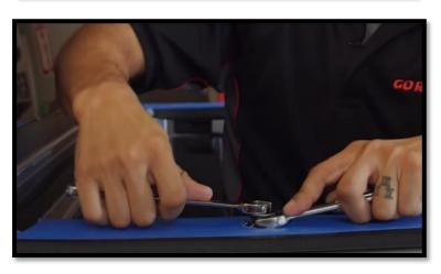
**STEP 15**: With the rivet nut positioned, use the provided rivet nut tool (item 25) to compress the rivet nut. Use a ¾" wrench to hold the spacer on the rivet nut tool and a 9/16" wrench to turn the head of the rivet nut tool. This will compress the rivet nut. Once tight, unscrew the bolt and repeat the steps for the remaining rivet nuts. **OPTIONAL**: You can use an impact gun on the head of the rivet nut tool or rivet nut gun to compress the rivet nut.
