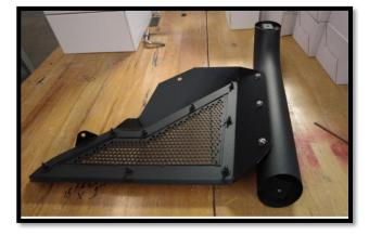
**STEP 3:** Attach front driver side tube (short) to the driver side mesh using ¼" button head screw (3), ¼" lock washer (3) and ¼" flat washer (3). Leave hand tight for later adjustment
