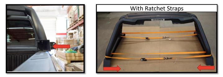
**STEP 9**: During adjustment, if the base plates overhang, you can use a clamp to secure it against the inside bed rail or use a pair of ratchet straps to keep it in place while adjusting it to your desired position.
