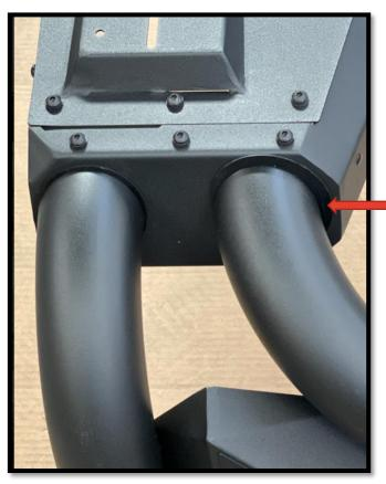
Verify that vinyl washer makes contact with the entire tube surface and center box to prevent metal to metal contact.
