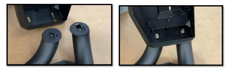
**STEP 6**: With assistance, install box assembly onto front and rear tubes as shown. Position the rear upper vinyl washer (item 14) and front upper vinyl washer (item 13) in between the tubes and base plate. Fasten down using 3/8" hex bolts (2), 3/8" flat washer (2) and 3/8" lock washer (2). Leave finger tight for later adjustment. Repeat steps for passenger side.
